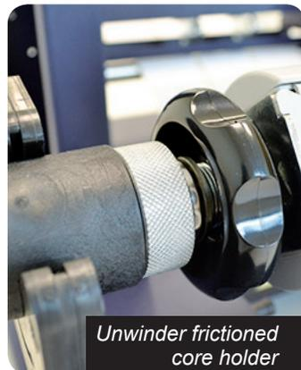
Unwinder frictioned core holder
